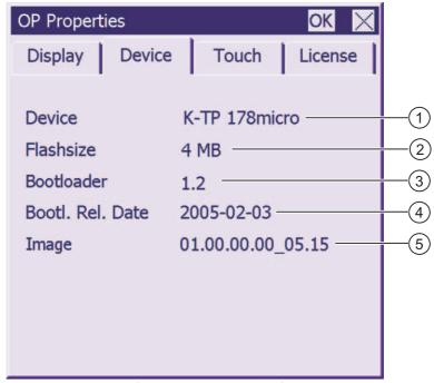
图 6-4 "OP属性"对话框,"设备"标签,实例
